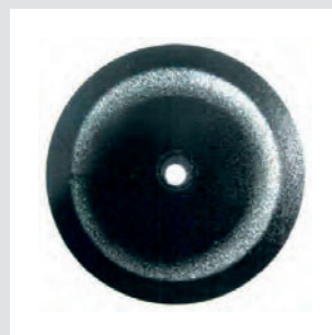
Abrasion test (loss of mass totaling 13.1 mg after 100 revolutions)
